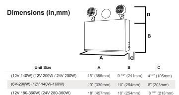
NOTE: Cabinet size may vary based on product configuration. Dimension D in drawing above will vary based on heads supplied. Cabinet size for 12V 160W Pb-A varies. Please contact factory for sizing information.
